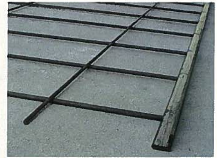
Fig. 5. Overall view of mesh and angle (M&A) connector (2 and 4 in. flanges). Note: 1 in. = 25.4 mm.
